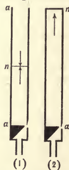
FIG. 156. — Nodes in Open and Stopped Pipes.
